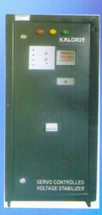
KALURIE™ range of Servo Controlled Voltage Stabilizers (SCVS) also known as Electro dynamic or Electro-Mechanical type of voltage stabilizer. These contain auto-transforme with servo-controlled motor for continuous voltage selection, with a feedback circuit. T accuracy of the output voltage is very high and is generally in the range of + or -1% for which these can be used for sensitive applications.
